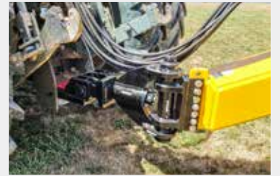
☛ A heavy duty drawbar is being used on this D10000.
