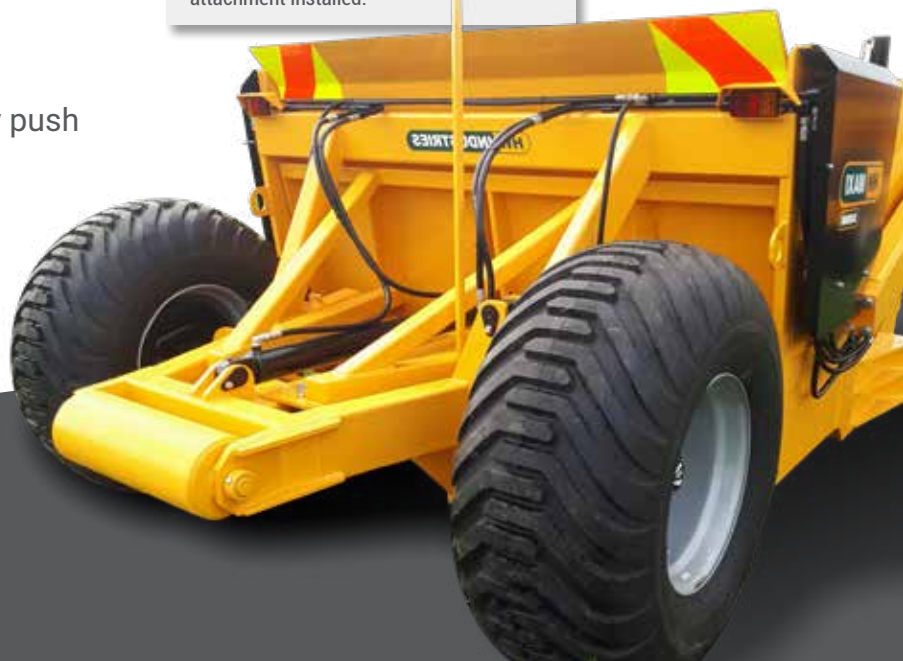
☛ This scraper has a push bar attachment installed.
