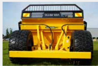
☛ This scraper has a push bar attachment installed.
