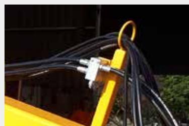
➤ This D8000 scraper has been fitted with a sequence valve.
