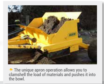
Being able to carry the load rather than dragging it you save wear and tear on the tractor/scraper and use a lot less fuel.
