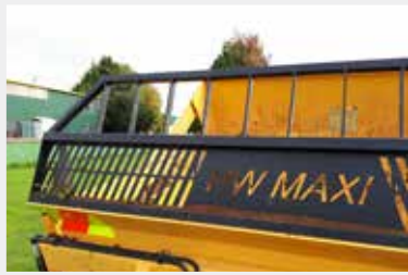
☛ A tailgate extension is being used to stop dirt spilling on this job.
