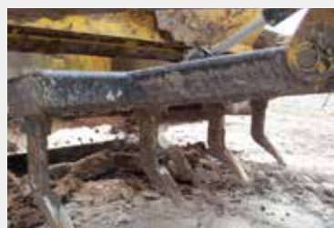
☛ Rippers are generally front mounted which allow you to prepare the ground and increase scraper efficiency.
