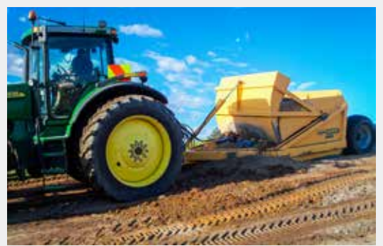
➤ A M800 being towed behind a 200 hp tractor to contour and create a sub-division.
