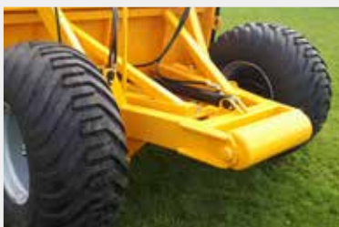
☛ This machine has a push roller attached for extended wear and increased efficiency on the job.
