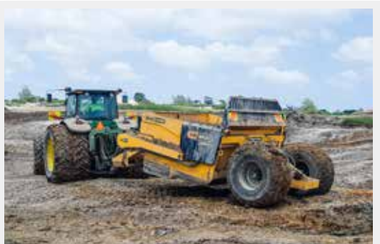
➤ A D10000 being towed by a 300hp tractor to spread soil over a paddock contour.
