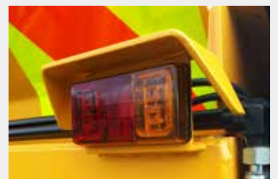
➤ A drawbar scraper fitted with tail lights for increased safety at night.
