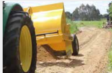
The unique design enables you to tilt the machine from side to side, allowing for beveled edges to be easily achieved.
