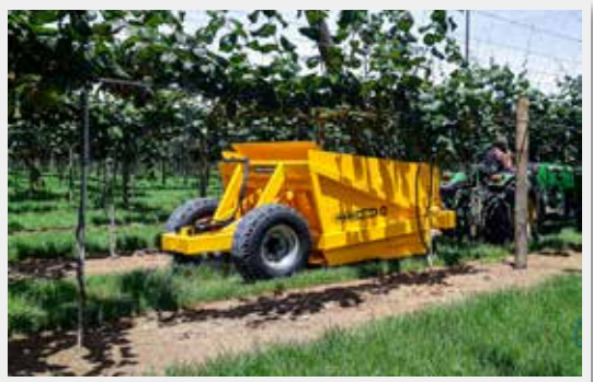
➤ A M300N scraper being used to shift dirt down an narrow orchard lane.
