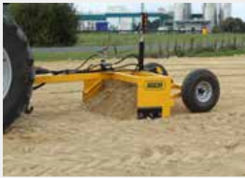
➤ This BX70 has a laser control system installed for increased efficiency.
